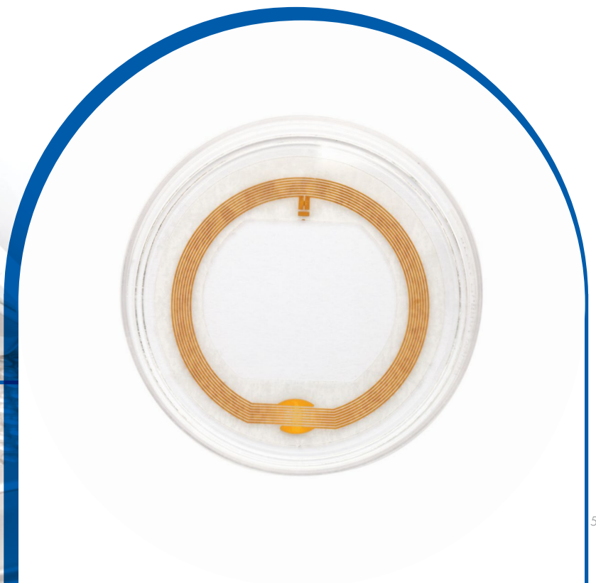
Self-adhesive RFID tag on Petri dish
